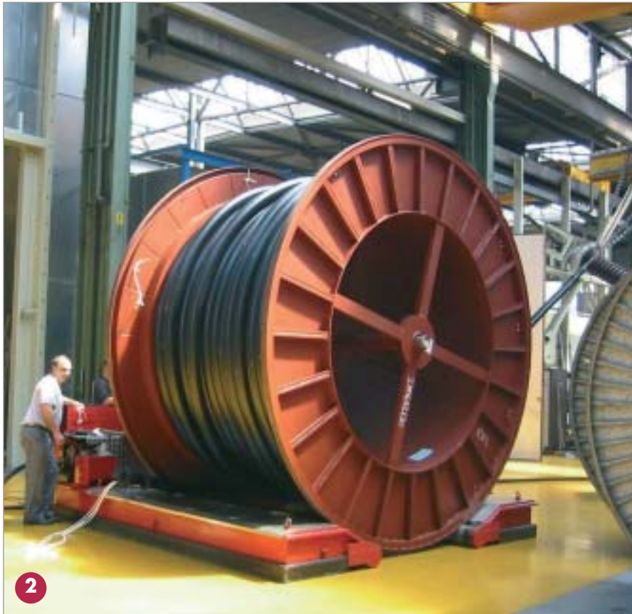
Air cushion system with cable roller
