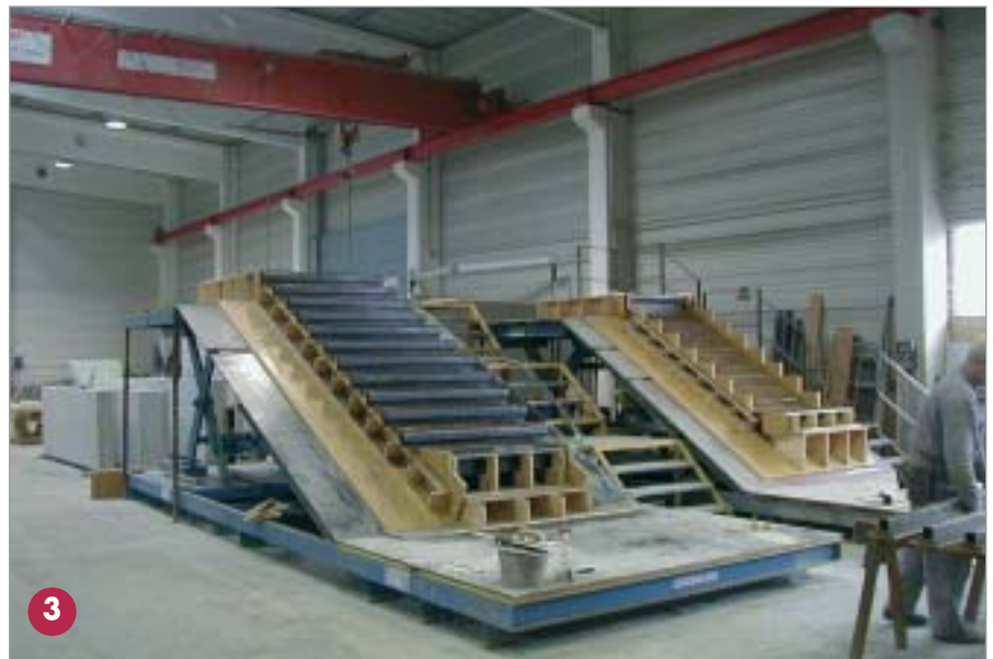
Shuttering ramp, stored on an air cushion system
