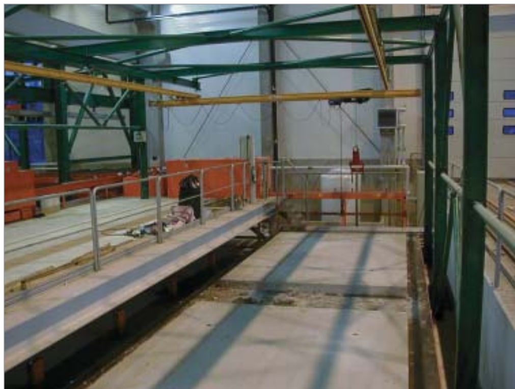
Solid element – early demoulding station
