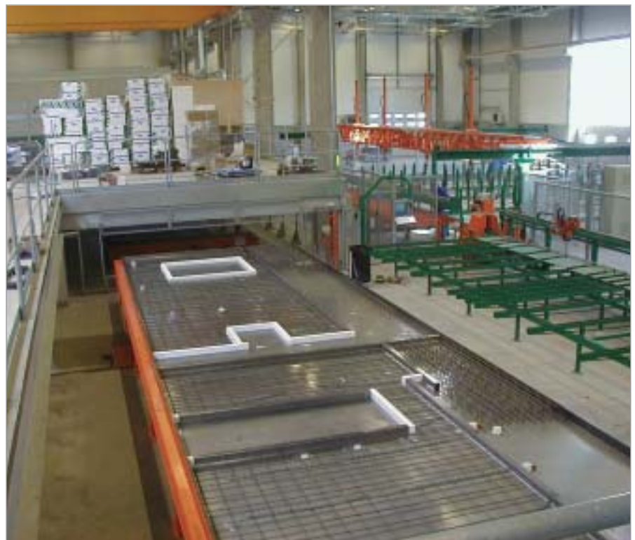
Processing the lattice girders
