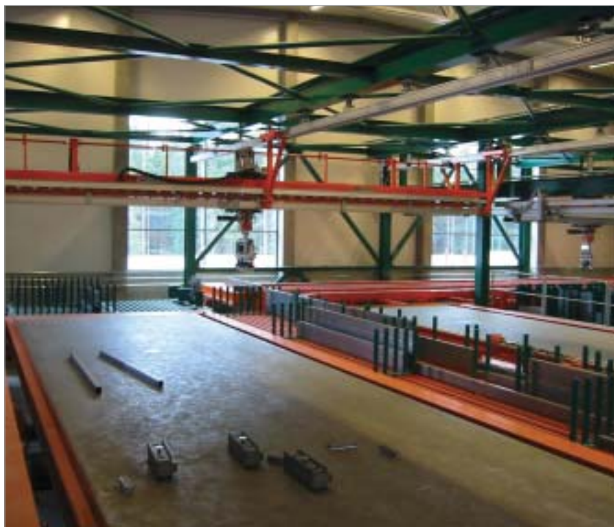
Shuttering robot and magazine robot during startup
