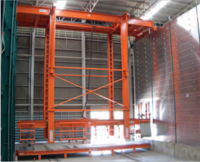
Rack operator and curing chamber
