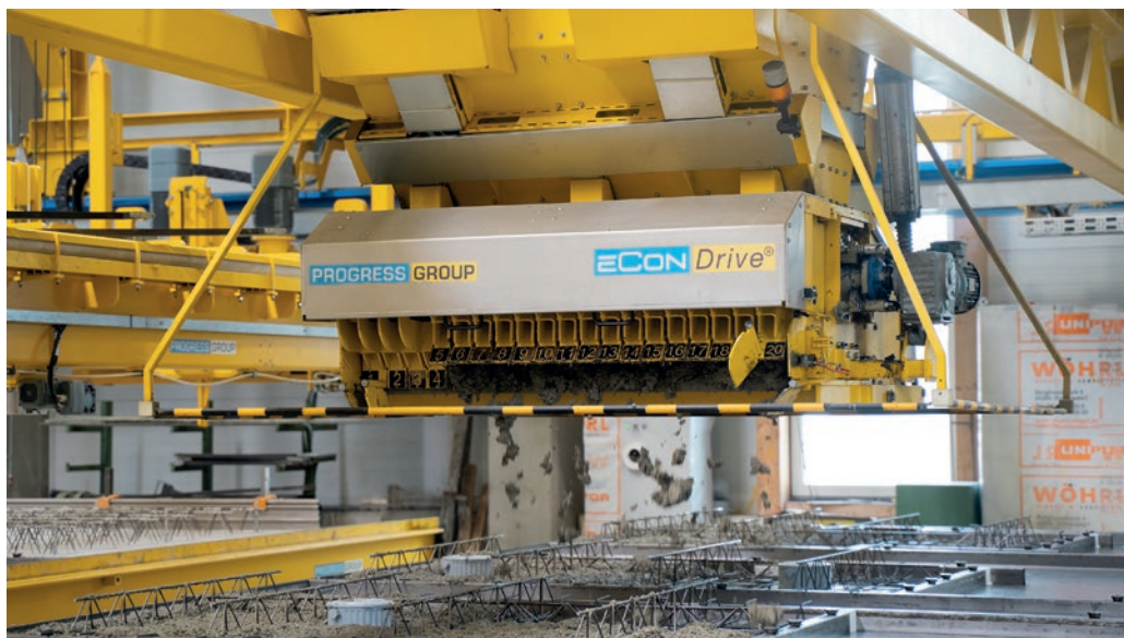
The eCon Drive concrete distributor is equipped with half-flaps, thereby achieving even more precise concrete discharge.
