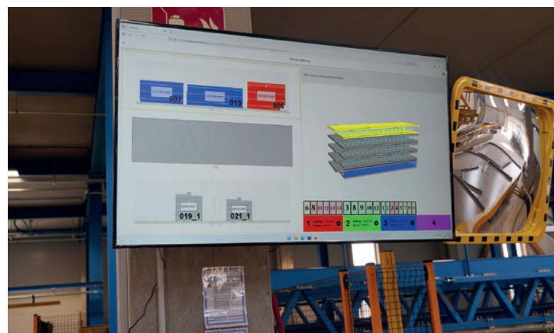
ebos yc controls the carousel plant and enables real-time monitoring and subsequent analysis through 3D visualisation. In addition, Smart Production Screens provide the necessary data at the optimum point in the production process.
