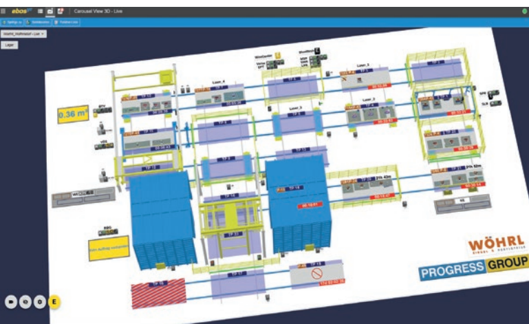
ebos yc controls the carousel plant and enables real-time monitoring and subsequent analysis through 3D visualisation. In addition, Smart Production Screens provide the necessary data at the optimum point in the production process.
