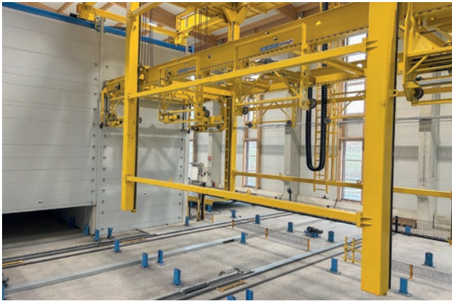
The most effective way to cure the elements is in a drying chamber. A storage and retrieval machine handles the fully automatic loading and unloading of the pallets.
