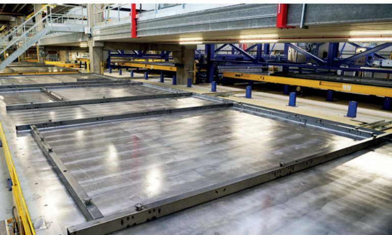
Fig. 6: Individual circulating pallets are transferred from line production into separate buffer locations ejected, separated by special vertically movable barrier fences
