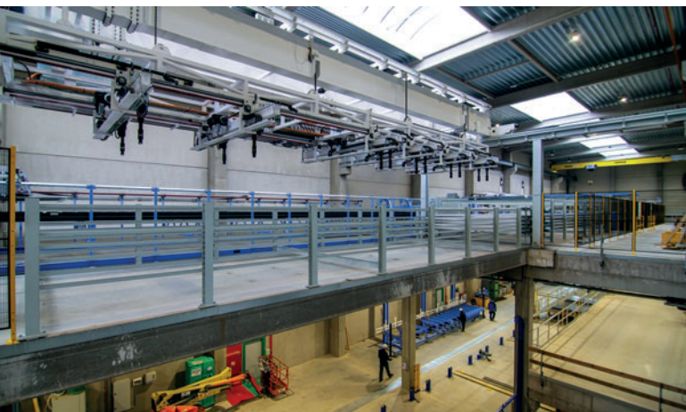
Fig. 5: The entire fully automated reinforcement preparation takes place on a higher intermediate level
