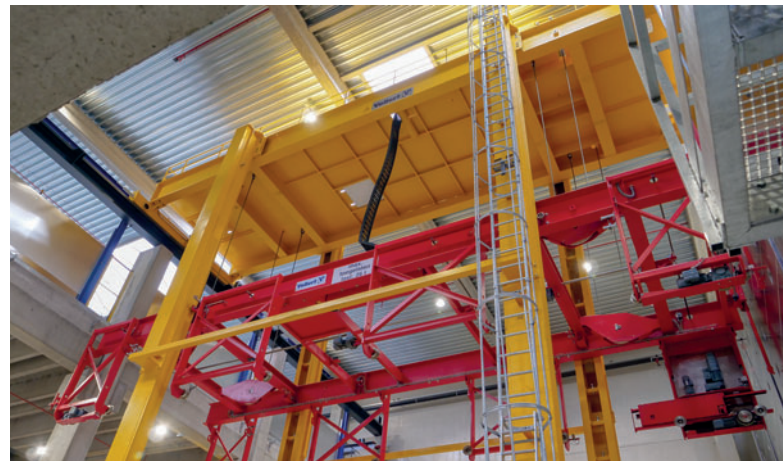
Fig. 8: On the intermediate level, the surface finish follows in a further development stage, directly served by the VARIO STORE storage and retrieval machine
