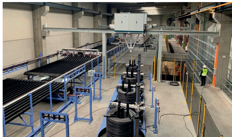
Fig. 5: The entire fully automated reinforcement preparation takes place on a higher intermediate level
