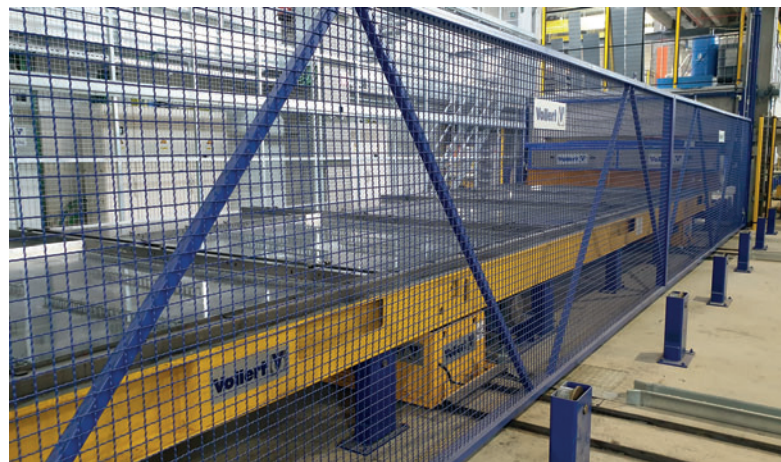
Fig. 6: Individual circulating pallets are transferred from line production into separate buffer locations ejected, separated by special vertically movable barrier fences
