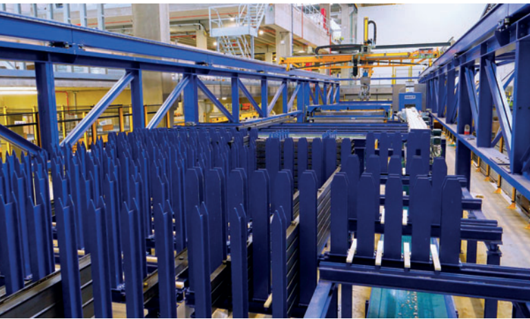
Fig. 4: The SMART SET shuttering robot also takes over the intermediate storage of the set-down profiles after the cleaning process in the storage racks
