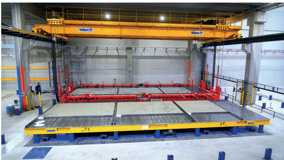
Fig. 9: Important technical innovations to increase cycle times and in the areas of ergonomics and occupational safety were realized at Kerkstoel 2000+ in double and sandwich wall production
