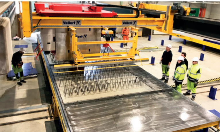
Fig. 7: A fully automatic, bridge-guided SMART CAST concrete distributor ensures optimum concrete cycle times and exact concrete dosing (Source: Kerkstoel 2000+)
