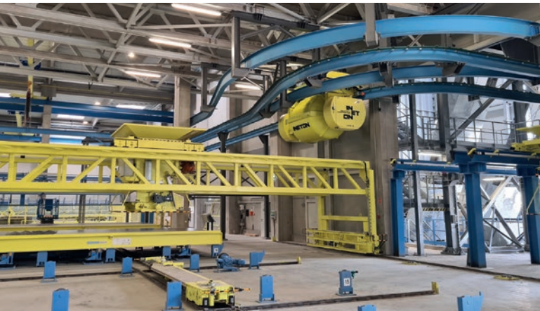
Concrete spreader and bucket conveyor system
