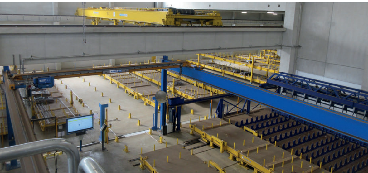
Loading of the transport pallets and transfer to the automated area
