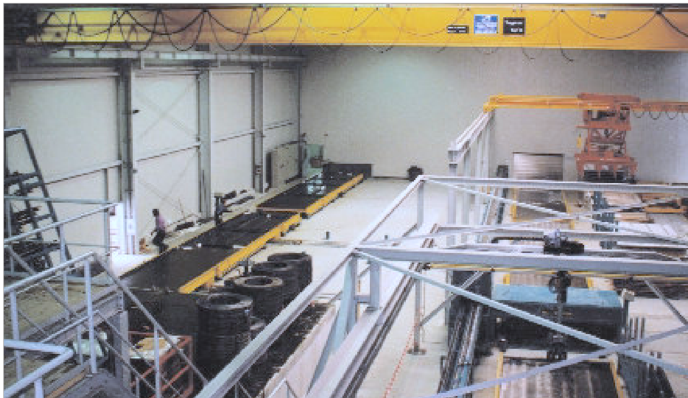
Production plant for slabs demoulding area and the mould-handling robots.
