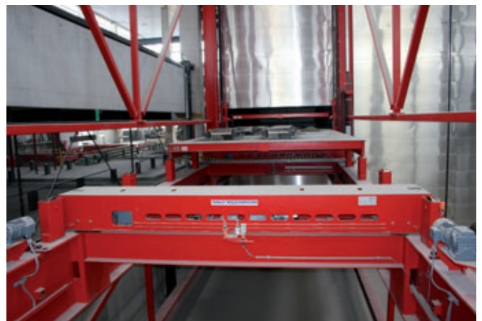
The storage and retrieval system services the 33 slots in the heated curing rack
