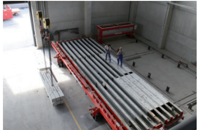
The formwork is stripped from the precast after being taken from the curing chamber and they are removed from the pallet by crane
