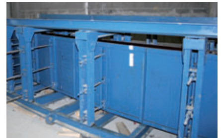
Formwork made by CTVS, a French manufacturer
