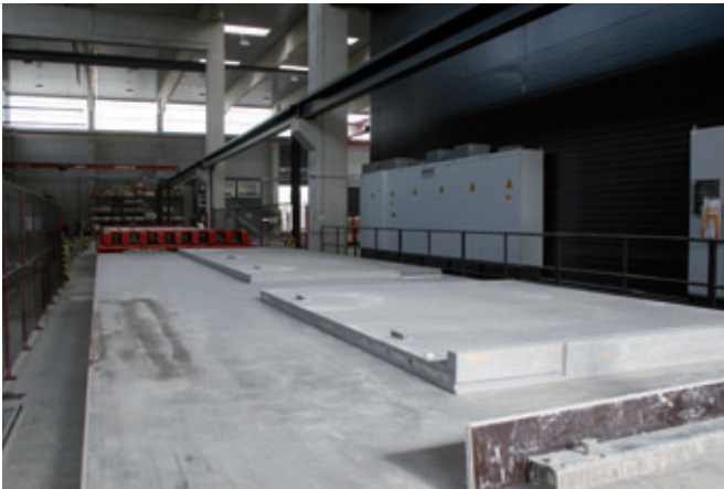
The formwork is stripped from the precast after being taken from the curing chamber and they are removed from the pallet by crane
