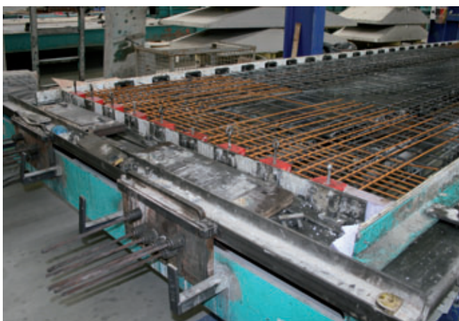
Formwork for ribbed flooring with untensioned and prestressed reinforcement
