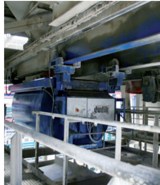
The concrete is distributed to the installation stations by a bucket conveyor system
