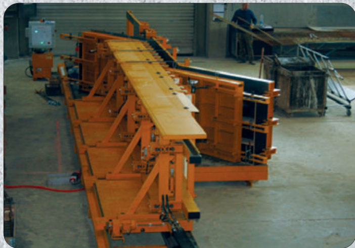
The concrete distributor spans the whole production area in the first hall.
