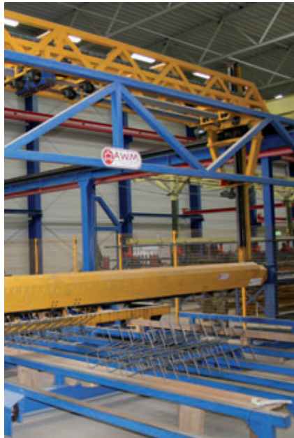
The automatic mesh bending machine in the front section of the hall for precision manufacturing of reinforcement
