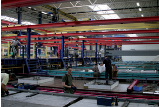
The workstations for wall production are each equipped with their own crane rail
