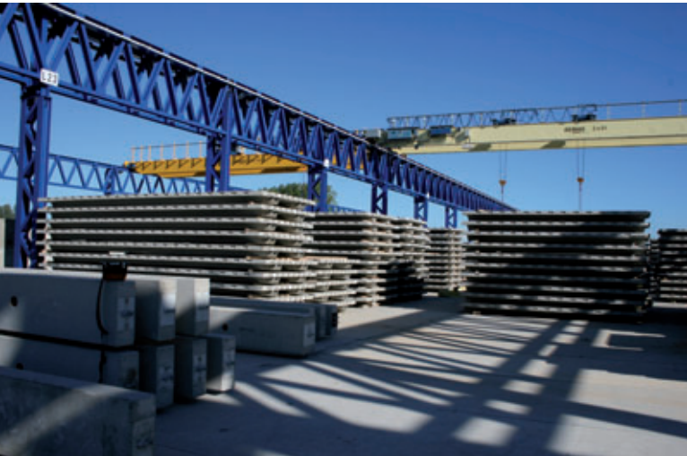
Ribbed flooring, whether untensioned or prestressed, is produced and stored individually for each project
