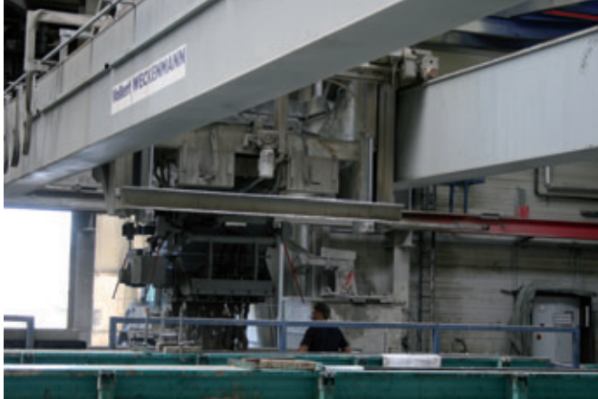
The concrete distributor spans the whole production area in the first hall.
