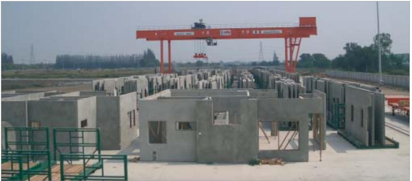
About 110,000 square meters of wall elements can be produced per month in this new facility
