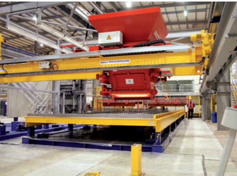
Fig. 9: Concrete Spreader and Compaction Stations
