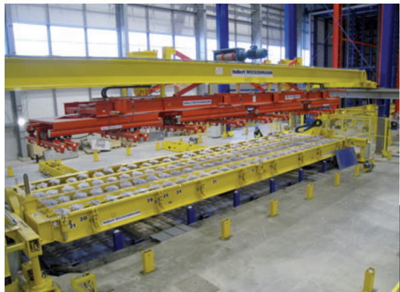
Fig. 12: Lifting and Vacuum Turning Device (During Assembly)
