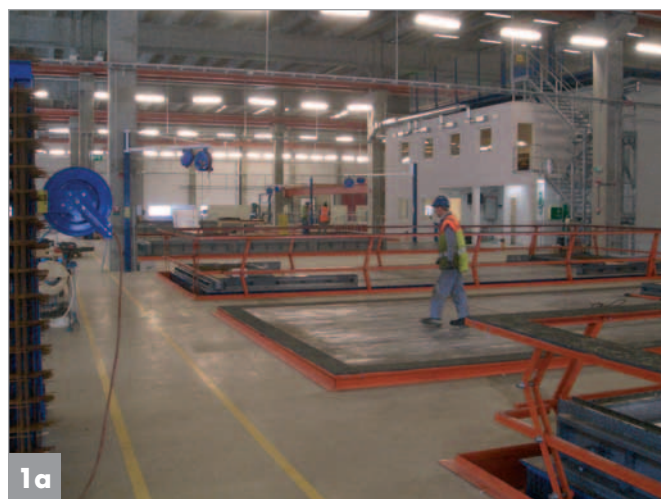
Placement of the side moulds, supported by a laser system
