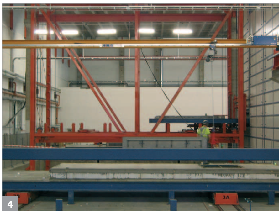
Storing of the pallets in the curing chamber
