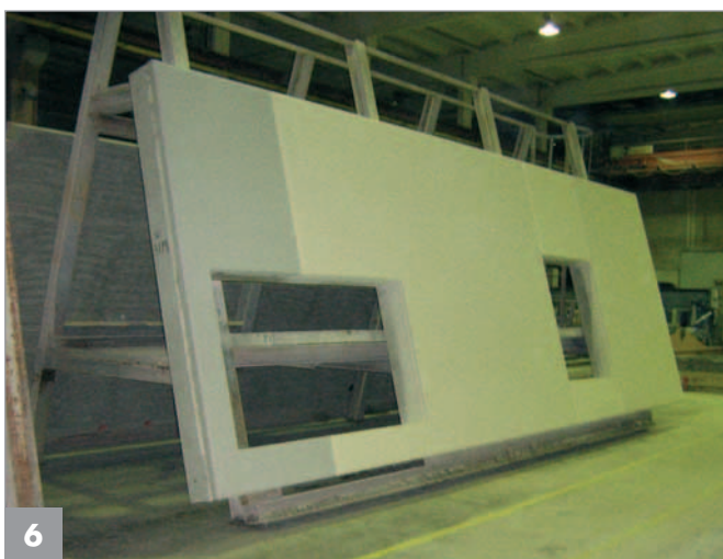
Finishing of the wall elements
