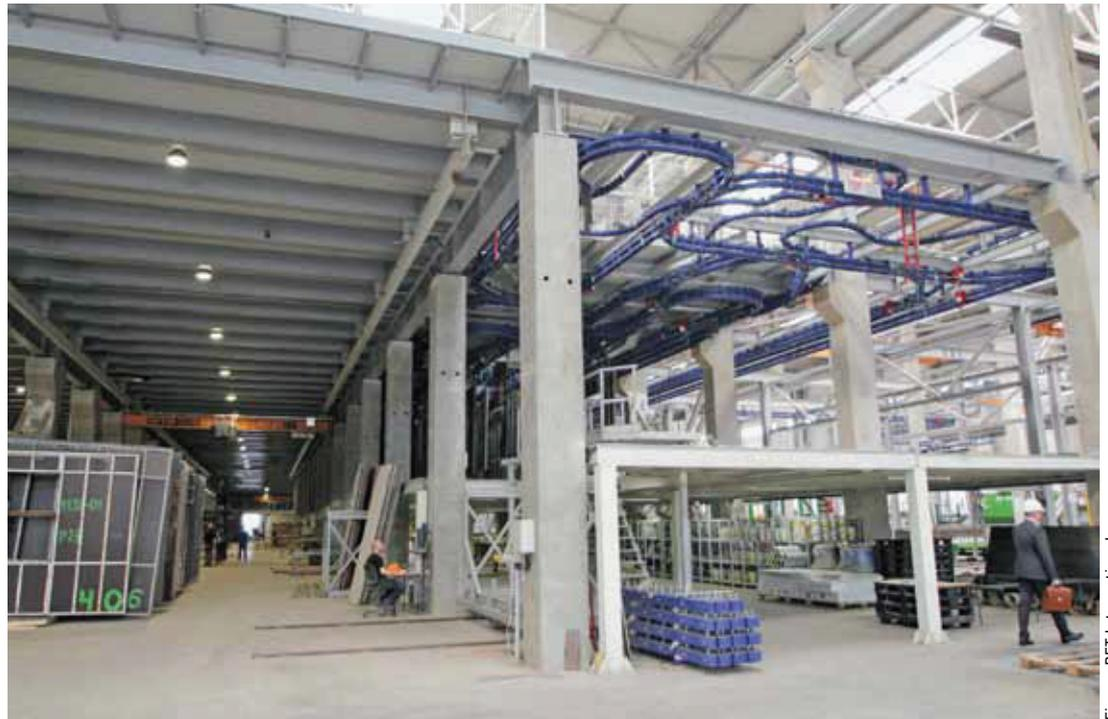
An automated handling system for formliners has been installed at the DSK Grad precast plant
