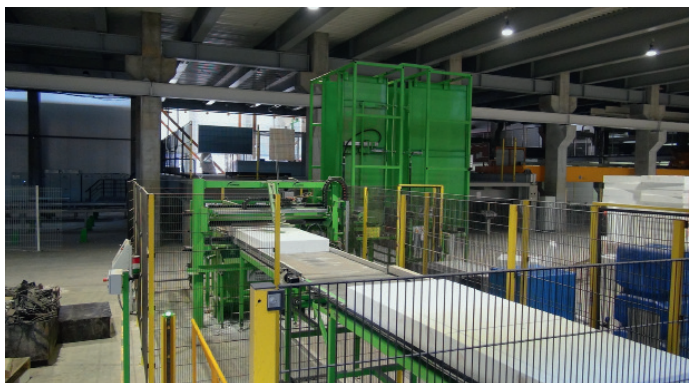
The innovative waterjet cutting machine cuts the polystyrene boards used for the insulation layer to size
