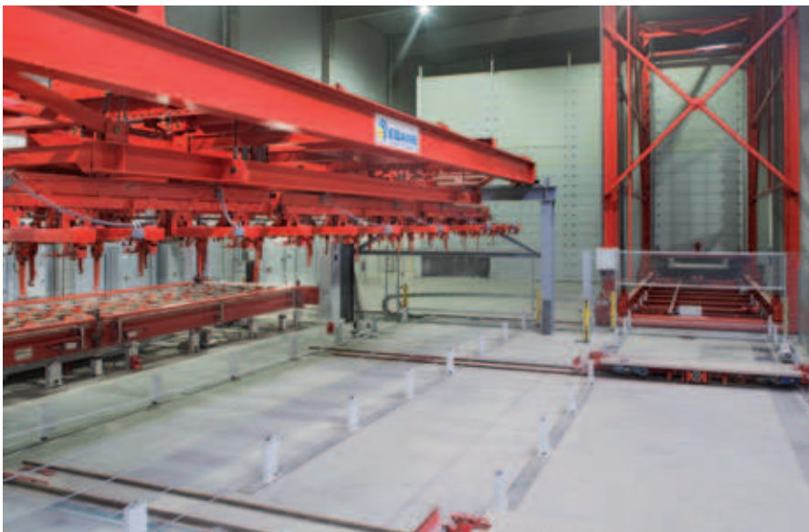
Picture of the double wall turning area
