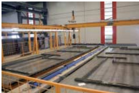
Fig. 8 The Shuttering robot works for two pallets; currently not needed shuttering elements are stored in the passive storage.
