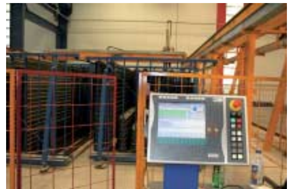
Fig. 8 The Shuttering robot works for two pallets; currently not needed shuttering elements are stored in the passive storage.
