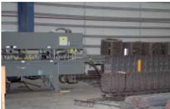
Fig. 11 Because there is no manufacturer for lattice girders in the Emirates, Mammut integrated an own lattice girder welding plant in its precast plant.
