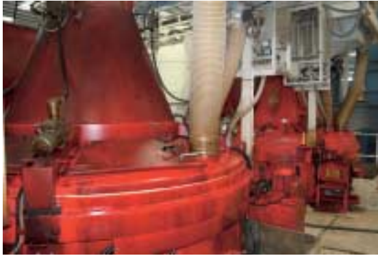
Fig. 2 Wiggert from Karlsruhe (Germany) installed two planetary Planetary counter-current mixers type HPGM 3000.
