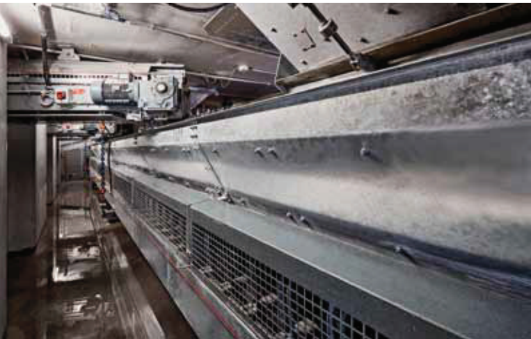
The material is transported by a withdrawal belt conveyor from the feed hopper into a bucket elevator
