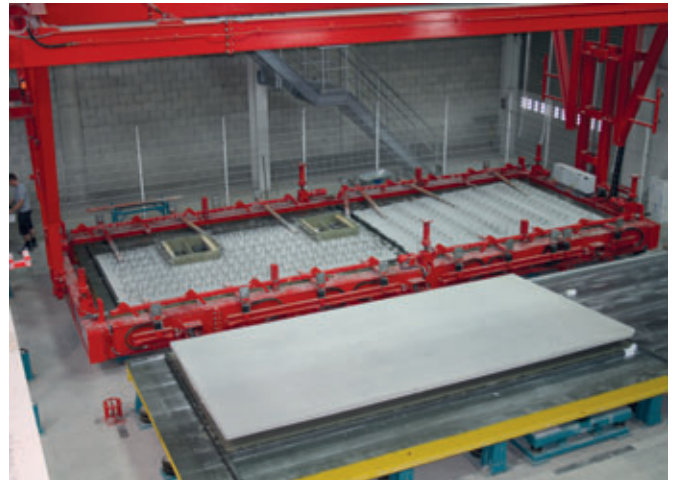
The hardening chamber with the storage and retrieval machine is located right next to the turning station
