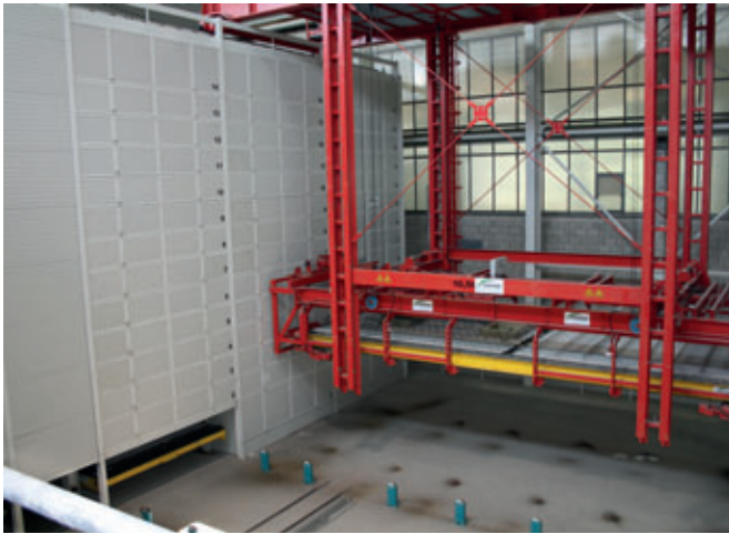
The hardening chamber with the storage and retrieval machine is located right next to the turning station
