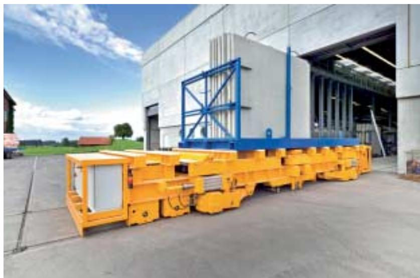
**Fig. 11** The produced elements are transported in the outside area with a specially designed exit carriage.
