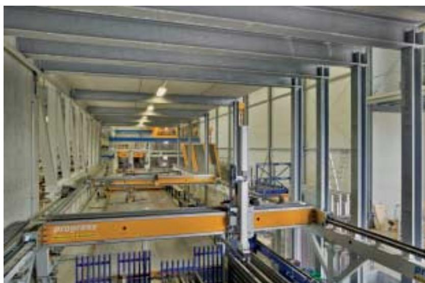
**Fig. 4** The shuttering robot does not only serve to move the molds onto the pallet but also to remove them: Molds are lifted from the pallet following a scan procedure. A second robot puts the cleaned molds in store again.
