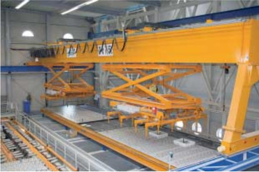
**Fig. 9** A special lifting device was designed for this unit: The system includes two lifting scissors fitted with four crossbars each. In turn, five load hooks are attached to each of these crossbars.
